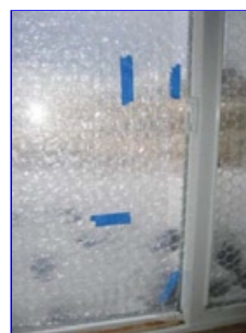
View through single and doubled bubble wrap. Blue tape is to take temperature readings on with the IR thermometer.
